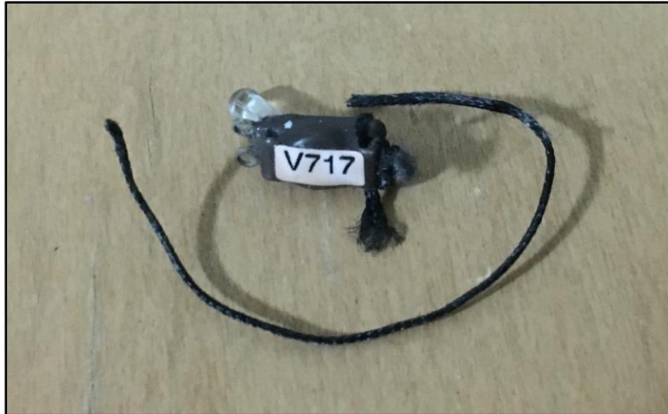
Figure 6. Sep-Dec 2015, Migrate Technology, Integeo-P50B1-7-dip, 0.55 g, 11-12 months estimated life. Unit V717, recovered October 7, 2016.
