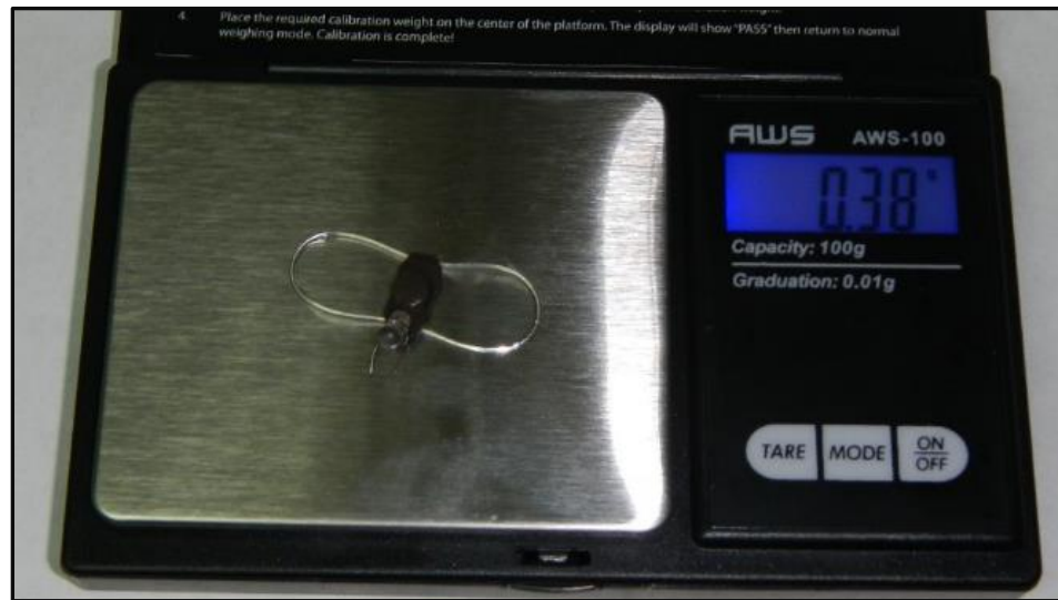
Figure 3. Migrate Technology Integeop-P30Z-7-DIP Light-level Geolocator with leg-loop harness attached, ready to be activated and deployed.
