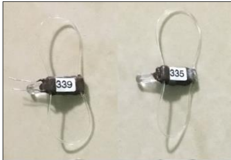
Figure 7. Unactivated Integeo-P30Z-7-DIP geolocator with uncut contacts (left, # 339), and activated unit with contacts cut and sealed with adhesive (right, # 335).
