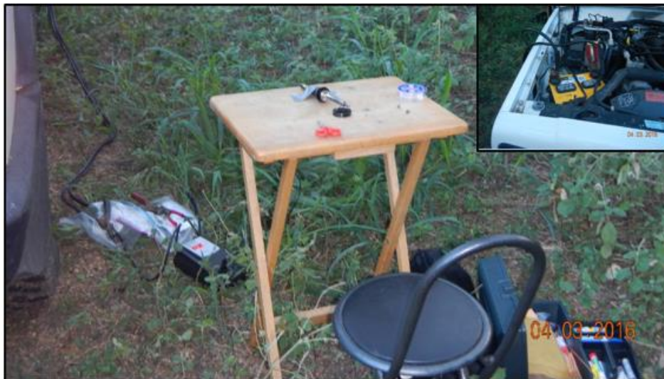
Figure 11. Field “mini-lab” setup for custom fitting of geolocator harnesses for individual birds, including a conventional soldering iron connected via an AC inverter to a vehicle battery.
