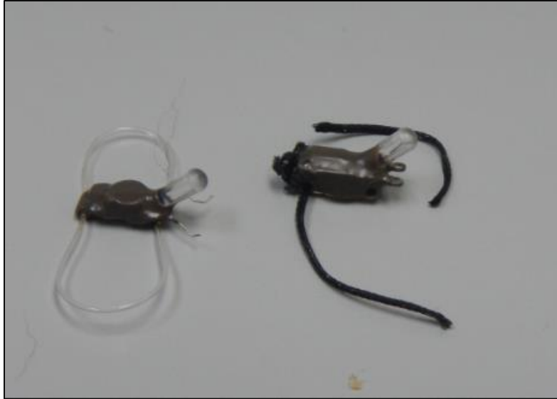
Figure 13. Comparison of the lighter model Integeop-P30Z-7-DIP (left) with the older model unit removed from bird 39307 on 28 Feb 2016.
