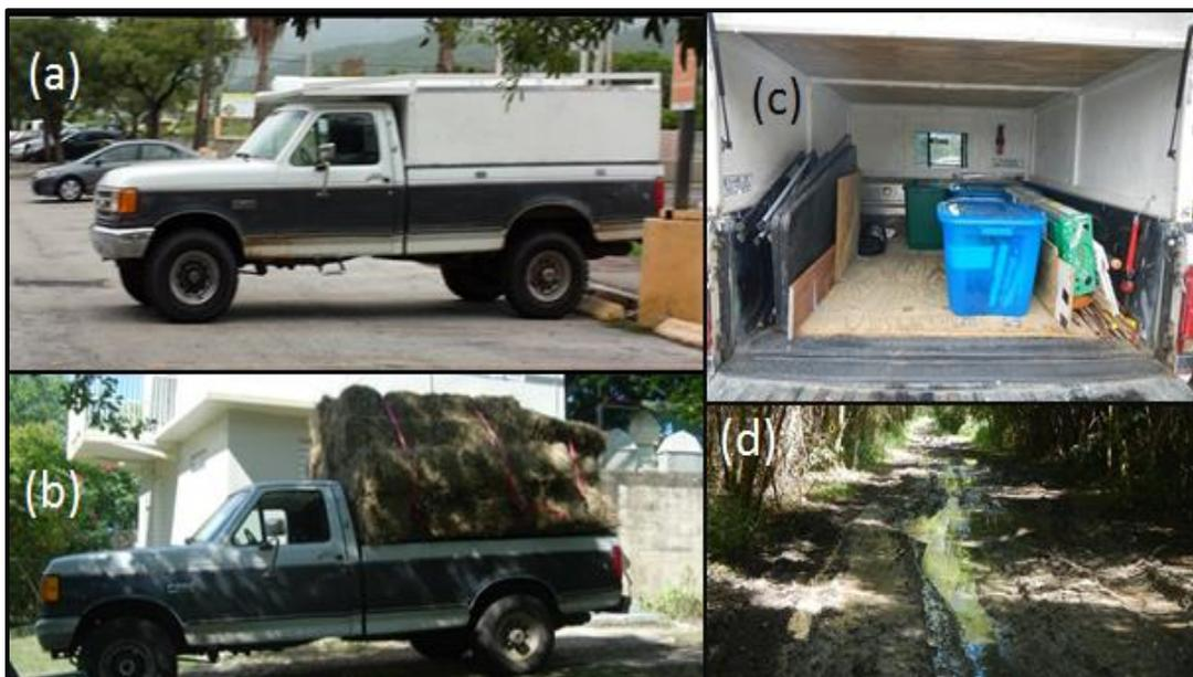
**Figure 4.** The project research vehicle, a 1991 Ford F-250. (a) The vehicle in its current configuration, (b) in its former configuration as a hay hauler, (c) interior, (d) road conditions to the study site during the rainy season. A six inch plastic sewer pipe (on the passenger side of the roof in (a)) is used to transport the 10-ft. galvanized EMT pipes used as net poles.
