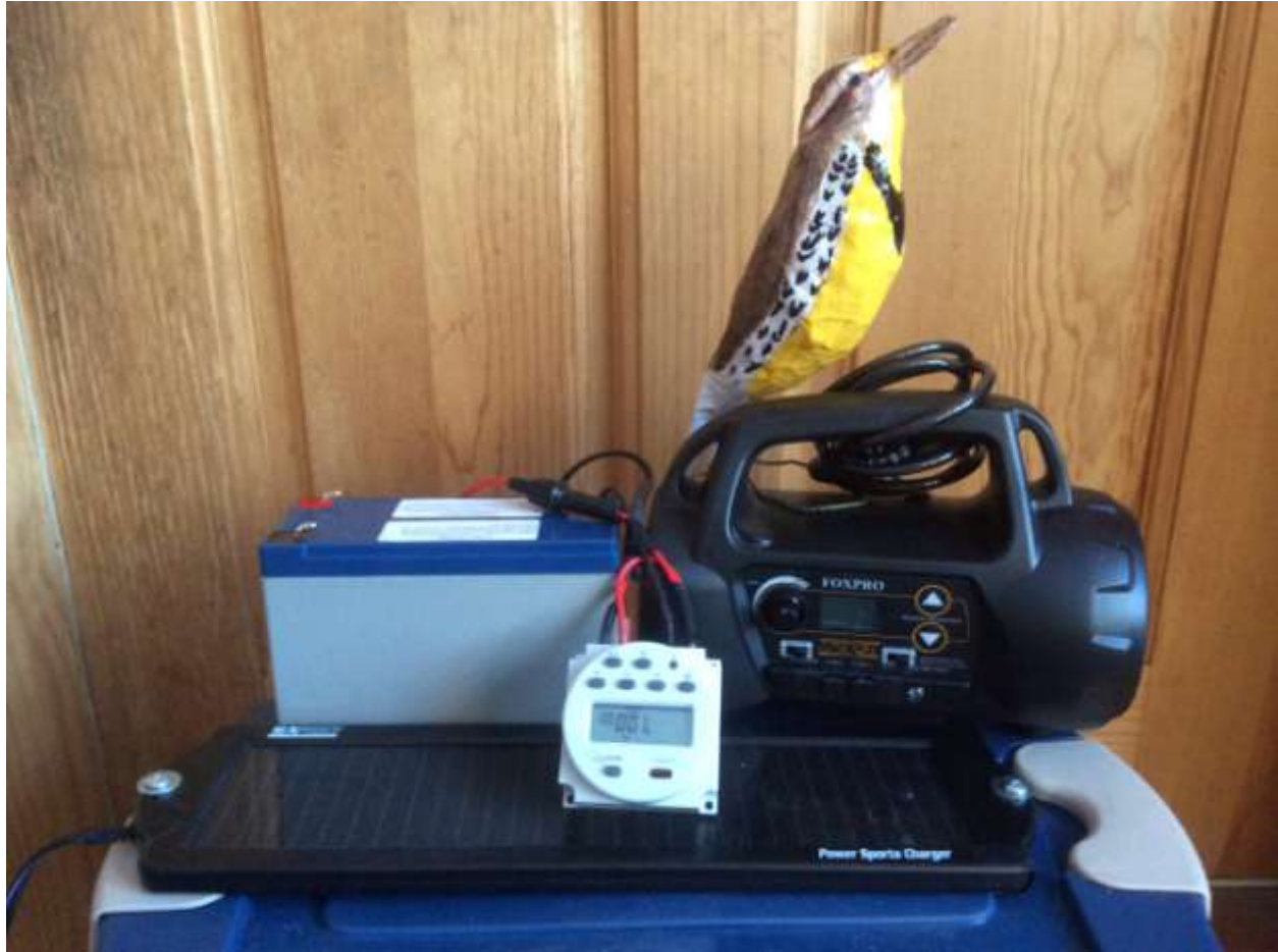
Fig. 1. Components of Eastern Meadowlark playback and decoy systems deployed at Daniel Webster and Allens Pond Wildlife Sanctuaries. Electronics were contained in waterproof plastic boxes mounted on 1.5 m high wooden standards.
